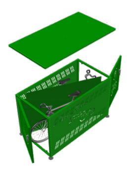
The Cycle Sitter provides secure, weather-resistant protection for your bike(s). Each bike nests in its own compartment with a separate locking door at each end of the locker (bi-directional access is required). With a user-supplied padlock, your bike and gear can be safetly stored away from prying eyes. Solid sheet and tubular steel construction with no exposed fasteners provides extra security.
