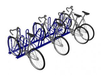
The Pinnacle-A Rack achieves high density bike parking by alternating the height for every other bike. The 8-1/2" height difference prevents the handlebars from contacting those of the next bike making it easier to park or remove bikes without damage. The Pinnacle-A Rack also provides superior security by including multiple locking points and excellent support for each bike. The rack itself is made from both heavy gauge steel and solid steel rod, further enhancing security and stability.
