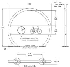
The Sunset Rack is constructed of heavy gauge, steel tubing and parks up to 2 bikes. It has multiple contact points for supporting the bike and locking the frame and wheel. The Sunset maintains a slim, appealing profile when not in use. The Custom Logo Plate can be provided with laser-cut graphics or as a blank plate suitable for vinyl graphics (applied by customer). The Logo Plate size can be adjusted to suit the logo or graphics.
