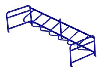
The Single Bike Stall fits 14 bikes in the space required for one car. Cyclists are separated from the flow of vehicular traffic by an end rack on either side of the stall.
