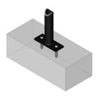
Base plates are anchored directly to the concrete using tamper proof anchors. Greenspoke includes the hardware required but there are several other hardware options also available. Typical anchor hardware: 1/2" security bolt
