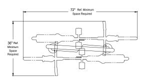
Top View Showing Recommended Spacing Requirements (/2 Scale)
