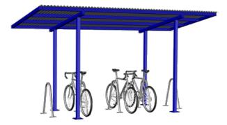
This 4 Post Shelter is designed to provide maximum weather protection for up to 12 bikes. The frame is constructed from rugged, tubular steel and the roofing panels are corrugated steel. This design provides superior stability and the modular system is simple to assemble. Columns can be anchored directly to a reinforced concrete pad or four separate concrete piers.
