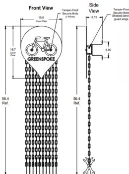
The Wall Mount Repair Station provides 9 of the most commonly required tools for road-side repairs or adjustments. The tools are safely secured on flexible tethers that are secured to a low-profile locking channel which is mounted to the wall.
