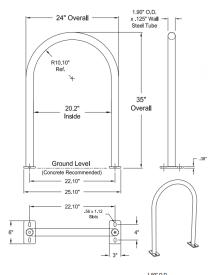
**FEATURES** Fully Welded Construction
