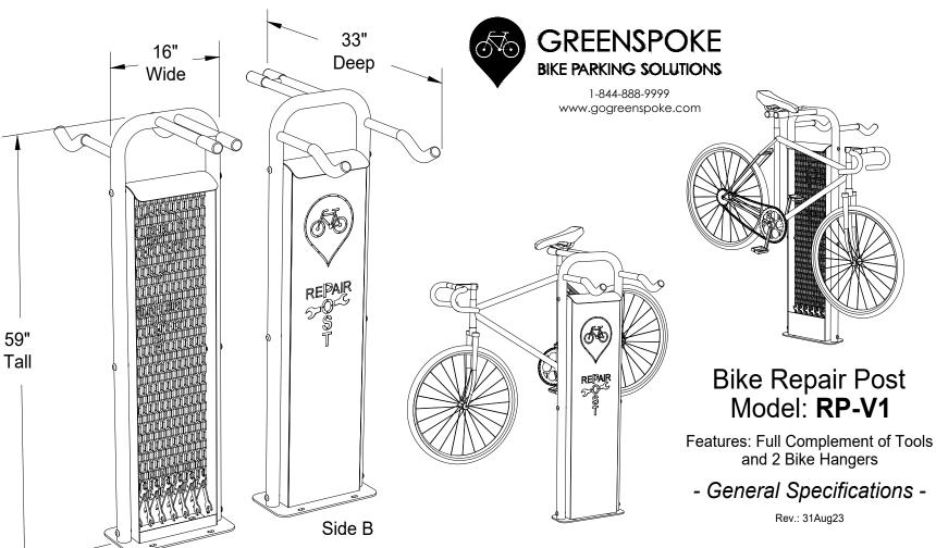
Ten of the most commonly required bike tools are provided, securely suspended from either Chain or Aircraft Cable.
