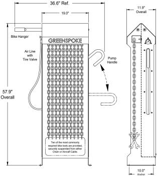
The RP-V5 provides a convenient place to perform roadside bike repairs or fill a tire, offering a selection of tools typically required for most bike repairs.
