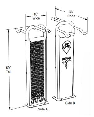
The Bike Repair Post includes a full compliment of the most commonly required tools. The tools are securely tethered with your choice of chain or coated aircraft cable.
