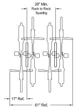
Minimum Rack to Rack Spacing (¼ Scale)
