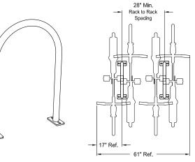
Minimum Rack to Rack Spacing (1/4 Scale)
