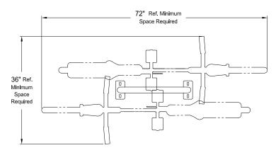
Top View Showing Recommended Spacing Requirements (½ Scale)
